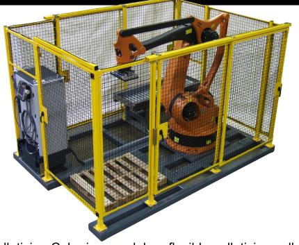
The P3 Palletizing Cube is a modular, flexible palletizing cell suitable for case, carton, pail and bag applications. The pre-assembled design results in an economical solution minimizing installation time and maximizing the return on investment.
